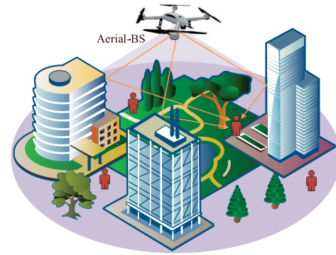
Fig. 1. The air-ground mmWave channels between the UAV aerial-BS and UD exhibit sparsity in both angle-domain and delay-domain due to the limited significant scatterers [25], [26].
