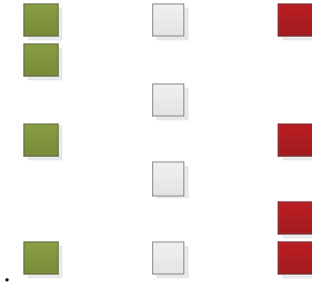
Fig. 3. Antenna-element distributions of the structured NURA in elevation domain given M_y = 4 : f_{0 < \alpha < 1(m)} (left), f_{\alpha=1(m)} (center), and f_{\alpha > 1(m)} (right).
