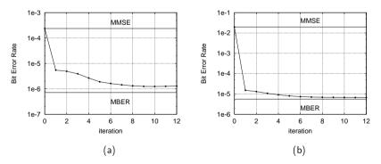
(a): SNR= 10 dB, SIR<sub>i</sub> = 0 dB for i = 2, 3, 4, 5, adaptive gain  $\mu = 1.0$  and  $\rho_n^2 = 6\sigma_n^2 = 0.3$ . (b): SNR= 10 dB, SIR<sub>3</sub> = SIR<sub>4</sub> = 0 dB, SIR<sub>2</sub> = SIR<sub>5</sub> = -6 dB, adaptive gain  $\mu = 0.5$  and  $\rho_n^2 = 2\sigma_n^2 = 0.1$ .
