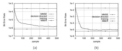
(a): SNR= 10 dB, SIR<sub>i</sub> = 0 dB for  $i = 2, 3, 4, 5, \mu = 0.03$  and  $\rho_n^2 = 8\sigma_n^2 = 0.4$ . (b): SNR= 10 dB, SIR<sub>3</sub> =SIR<sub>4</sub> = 0 dB, SIR<sub>2</sub> =SIR<sub>5</sub> = -6 dB,  $\mu = 0.02$  and  $\rho_n^2 = 4\sigma_n^2 = 0.2$ .
