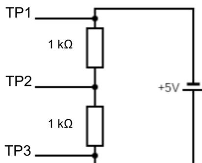
3. Connect the voltmeter to measure the voltage between test point 1 and test point 3. Note down this supply EMF into table 1 below.
