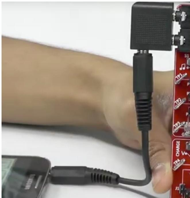
3. Connect the output of the Music Mixer circuit board to the oscilloscope using a 3.5mm plug to bare wires cable. Connect the oscilloscope probe to the bare wires. The main part of the probe should clip onto the red coloured wire, and the crocodile clip should connect to the black wire.
