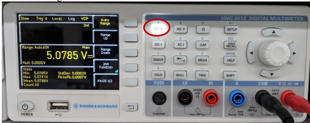
Figure 2. Image of the benchtop multimeter showing the configuration to measure voltage.
